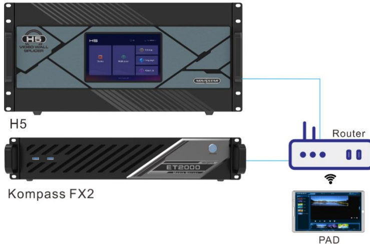
Figure 6-5 Connections for App control
