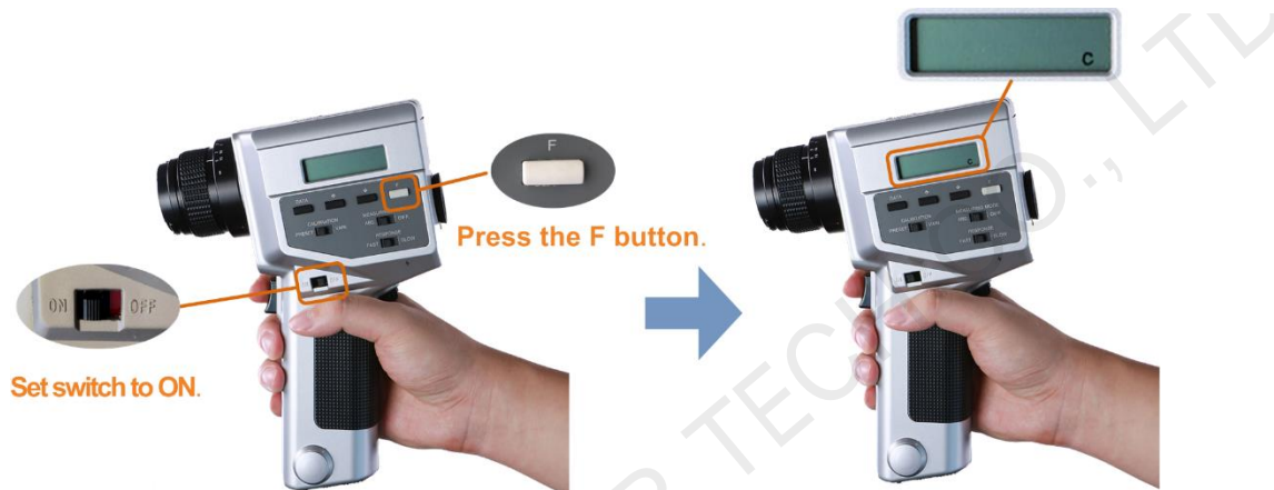
Figure 12-7 Setting CS-100A colorimeter
